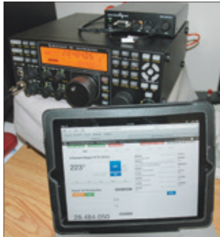
The RemoteHamRadio K3/0 with the Remote Rig interface and the Apple iPad 1 was using at the time.
